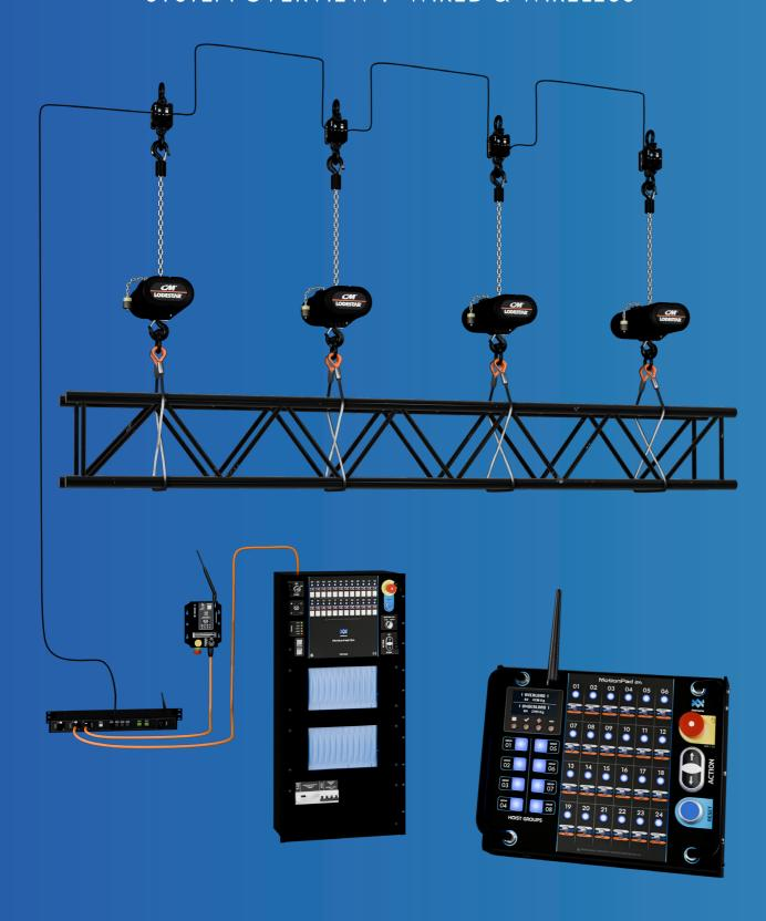
Our load cell system shares the same philosophy as our range of digital controllers, being able to work with cable connection only, fully wireless, or a mix of both.
