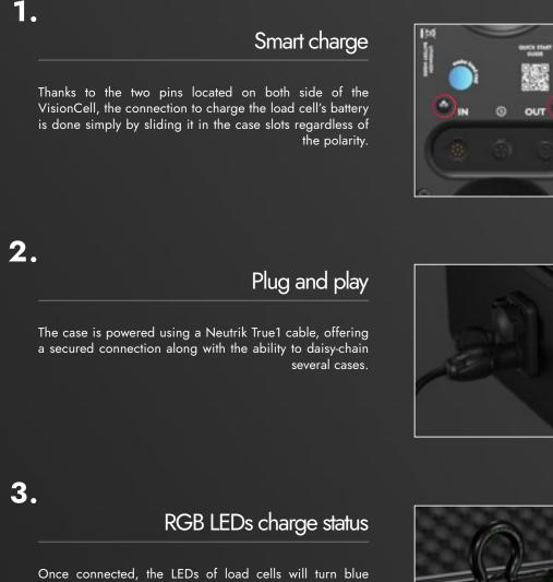
Once connected, the LEDs of load cells will turn blue to confirm that the charging is in progress. When fully charged, the LEDs will be lit in green, allowing you to make sure your system is ready at a glance.
