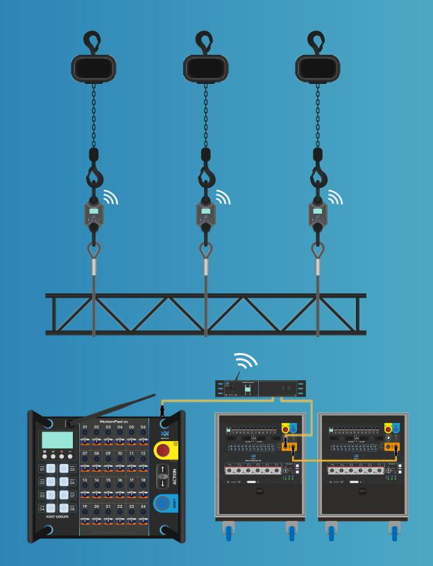
This other configuration above shows our load cells using wireless transmission to communicate with the receiver, while the two controllers are linked and operated using a wired remote.
